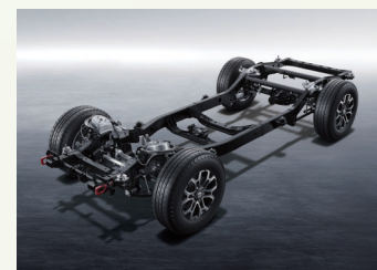
Separate frame constructure
